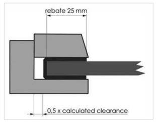
Sealing material must allow the movement of sheet inside the profiles due to dimensional changes of sheet. Profiled EPDM joints, preferably in white, have proven to be successful in heat loss avoidance. In most cases, profiled joints of non-rigid PVC and PUR foam are incompatible, due to the migration of plasticizers.
