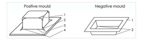
Negative forming means that the semi-finished sheet is drawn into the mold cavity. This is sometimes called "female" forming
