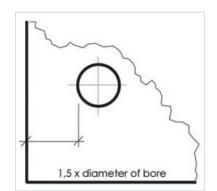
The drilled holes must be adequately dimensioned when fixing to specific points, in order to allow a sheet length clearance of 5mm/m, too.
