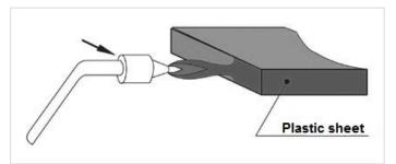
Improved surface finish is achieved by treating the sawn edge with an iron scraper prior to flame polishing.
