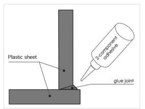
**Polymerization adhesives** are also suitable for large and uneven bonding surfaces. Planar bonding is possible.
