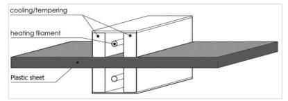
It must be possible to bend the material under low strain in order to avoid strong stresses in the material. The bend radius must be twice as big as the material thickness in order to prevent wrinkles and high stresses.
