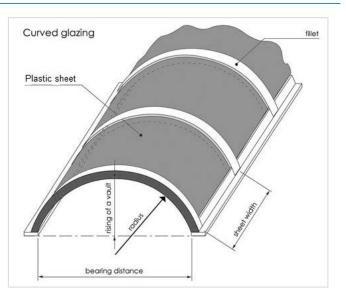
Recommended material thicknesses in mm at a given surface load of 750 N/m<sup>2</sup> can be obtained from the following table.
